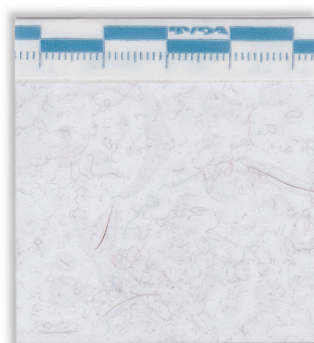
Hairs and fibres sampled with a transparent Instant lifter
